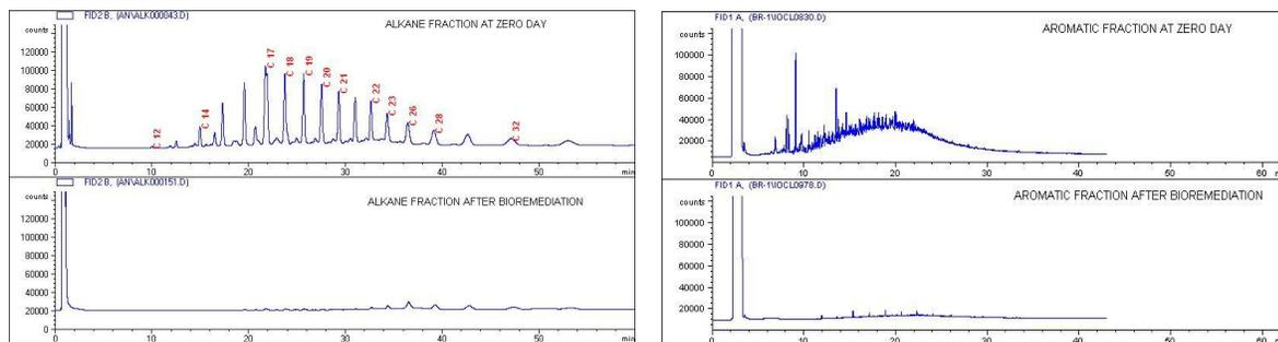
Figure 3 : GC chromatogram indicating the biodegradation of alkane and aromatic fraction of TPH at CPF Gandhar, ONGC, Ankleshwar Asset, India.
