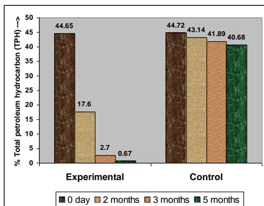
Figure – 2: Biodegradation of TPH of oil contaminated soil at CPF Gandhar, ONGC, Ankleshwar Asset, India.
