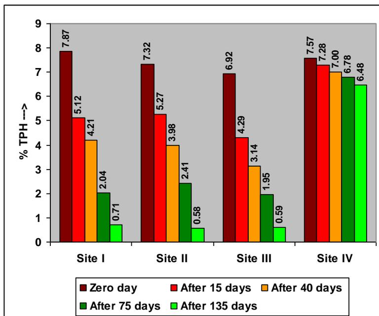
**Figure – 1: Biodegradation of TPH of oil contaminated soil at South Santhal CTF, ONGC, Mehsana Asset, India. Site – I, II & III are experimental sites and Site – IV is control site where no Oilzapper was applied.**
